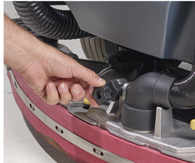
7. Check the height of the squeegee by adjusting the castor wheels and the angle knob.
