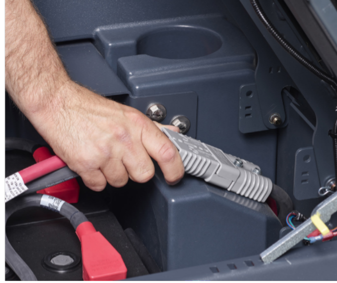
3. Check battery cables are well connected together
