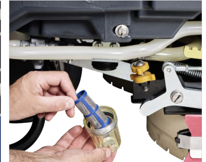
10. If necessary open the solution filter cage and clean the net.
